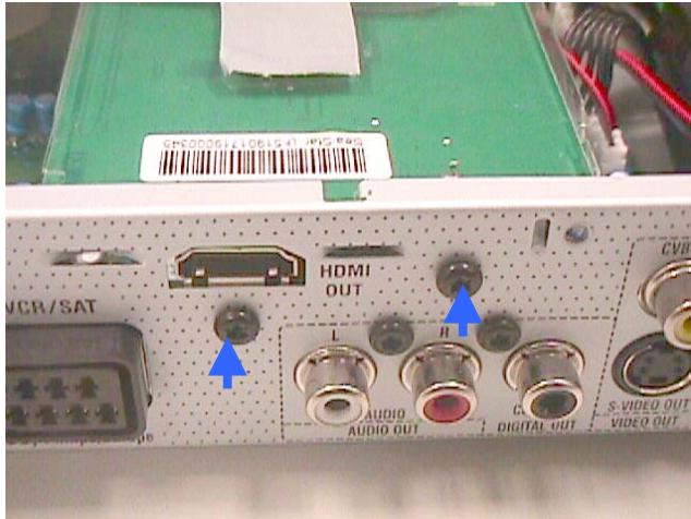
Figure 11 – HDMI Board mounting screws
